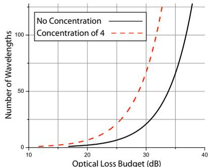
**Figure 6. Insertion loss analysis of Photonic Torus topology.****Table 3. Optical Device Parameters**
